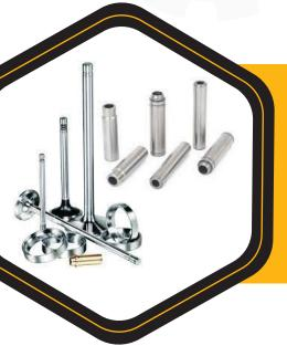
GREY CAST IRON of perlitic structure with high phosphorous content. The perlitic structure and the reticular phosphide distribution along with the good graphite formation give high wear resistance and improved running properties in poor lubrication condition.
